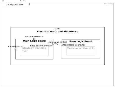
Electrical Parts and Electronics «HW» C0019 (appears in Section 1.5.1: L2 Mechanics, Section 1.4.3: L1 Physical View, Section 1.4: Solution Strategy, Section 1.5: Building Block View, Section 1.5: L2 Electric Parts and Electronics)
