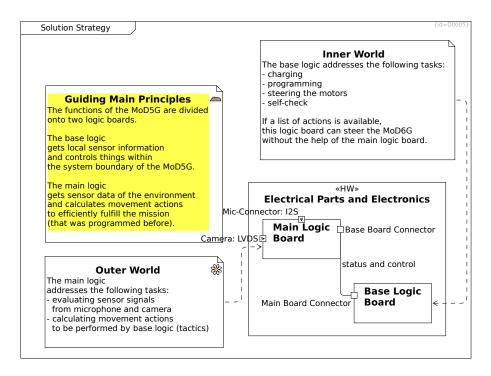
**Electrical Parts and Electronics** «HW» C0019 (appears in Section 1.5.1: L2 Mechanics, Section 1.4.3: L1 Physical View, Section 1.4: Solution Strategy, Section 1.5: Building Block View, Section 1.5.2: L2 Electric Parts and Electronics)
