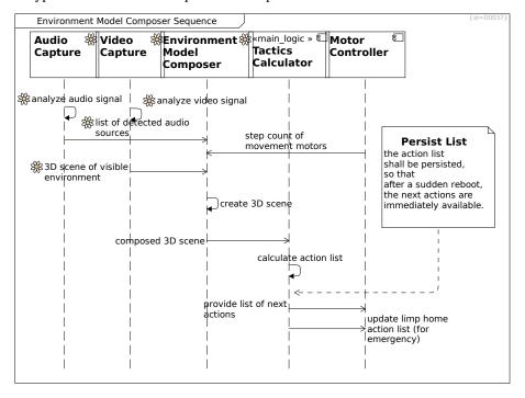
**Motor Controller** C0109 (appears in Section 1.5.3.6.1: Environment Model Composer Sequence, Section 1.5.3.5.2: System Control, Section 1.5.3.5: Building Block View, Section 1.5.3.7: Deployment View)
